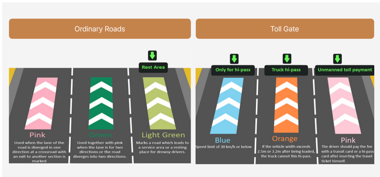
Figure 3 Classification of Road Surface Color Guide Lines for Ordinary Roads, Expressways and Tollgates
